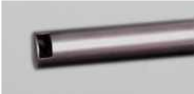
ASME PTC 4.2 sample nozzle
