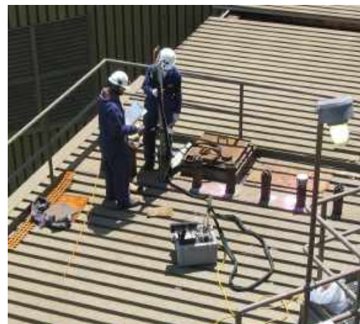
EPA Method 2 testing in a flue gas duct using the S-Type pitot probe
