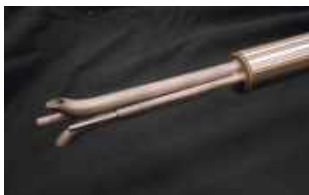
Pressure-sensing head for clean air pitot (S-Type)
