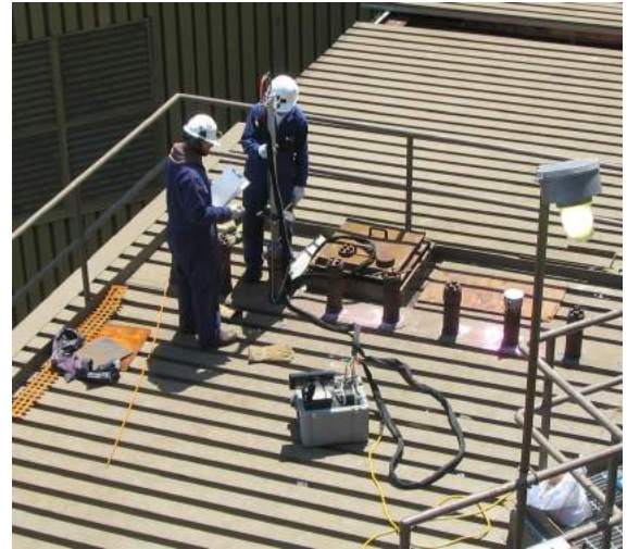
EPA Method 2 testing in a flue gas duct using the S-Type pitot probe
