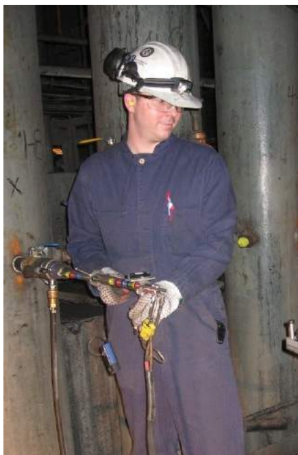
Velocity testing in a coal piping system
