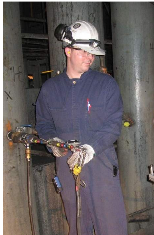
Velocity testing in a coal piping system
