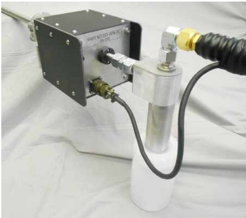
Motorized SwivelSampler, cyclone separator, sample jar, and umbilical
