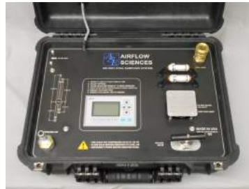
Control panel with PLC controller
