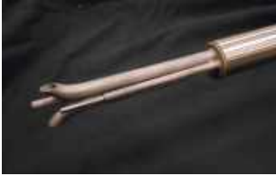
Pressure-sensing head for clean air pitot (S-Type)
