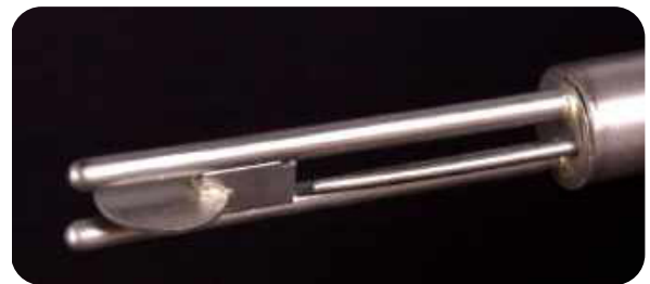
DAP probe sensing tip - custom designed for minimal particulate plugging
